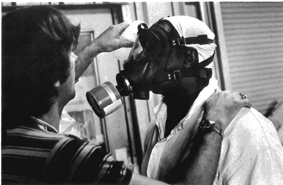
Fig. 17. On the basis of the Laboratory's extensive research on respirators, Los Alamos personnel were requested to observe and evaluate the protection provided to workers involved in the cleanup at Three Mile Island. The Laboratory had tested most of the respirators in use there for effectiveness against inhalation of radionuclides, particularly iodine isotopes, and has developed techniques to assure their proper use. Here a respirator is being checked for leaks with a strong smelling solution known as banana oil. (Photo by Alan Hack.)
