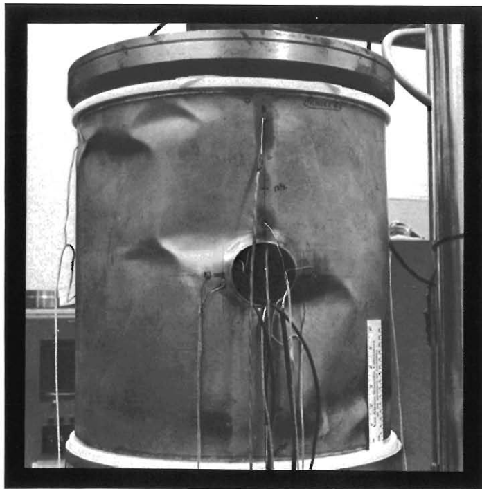
Fig. 5. One of the steel cylinders used in the simulated tests of containment shell buckling. The central hole is a scaled representation of the penetration for personnel and equipment access. In this case, the penetration has been reinforced inside the cylinder to 33 per cent of that recommended by the ASME code. Considerable buckling is evident around the hole. The small wired devices attached to the cylinder on both sides and above the hole are strain gages. Other gages are attached on the sides and back of the cylinder and at the same positions inside.
